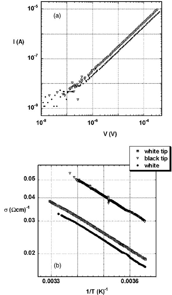
FIG. 1. Transport data collected from the ampullary gel of sharks: (a)  $I$ - $V$  traces show Ohmic response at various applied potentials, up to (not shown) 1 V; (b) semilog plot of conductivity vs reciprocal temperature for all three species. Range of temperatures matches range of possible environmental temperatures encountered by elasmobranchs (roughly  $0$ - $30^\circ\text{C}$ ).
