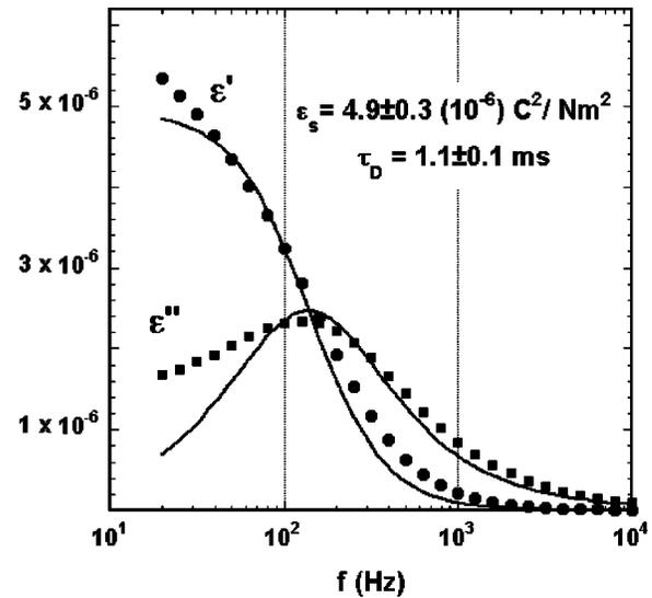
FIG. 2. Real and imaginary permittivity plotted vs frequency. The frequency-independent geometry factor was determined via an empty cell calibration assuming  $\epsilon_0$  for the permittivity of air. For our low-frequency experiments, the high-frequency permittivity,  $\epsilon_\infty$ , was set to that of water.
