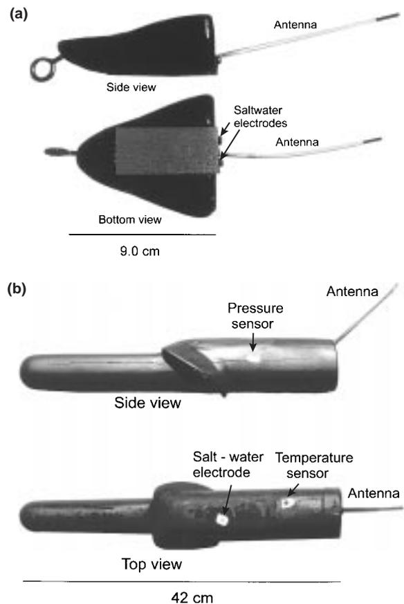
Figure 2. Towed satellite-linked radio transmitter designs used in whale shark tracking: a - type I instrument as viewed from the side (upper) and bottom (lower). b - type II instrument as viewed from the side (upper) and top (lower).
